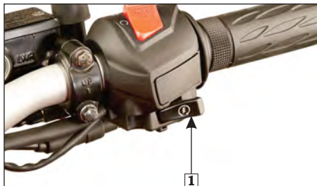
(1) Electric starter switch
