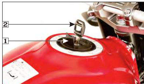
(1) Key hole cover (2) Ignition key
