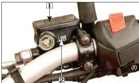
(1) Master cylinder/Reservoir (2) Lower mark
