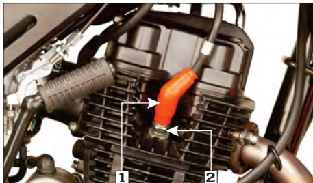
(1) Noise suppressor cap
