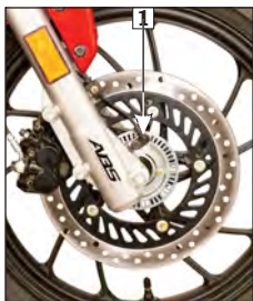
(1) Wheel speed sensor
